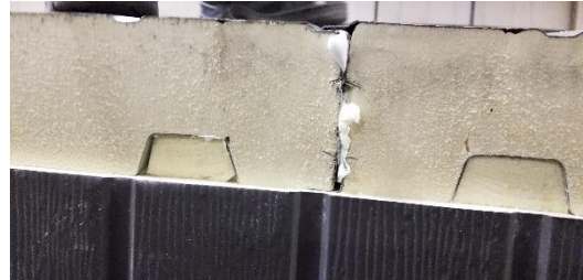
Figure 51: Acceptable Joint with proper squeeze out
