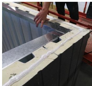
Figure 45: 1" polyurethane sealant bead 1 1/2" in from outside
