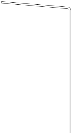
192615(X1) 2 1/2" X 4 1/2" X 90" FRONT ROOF ANGLE
