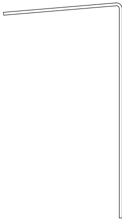
192616(X1) 2 1/2" X 4 1/2" X 90" BACK ROOF ANGLE
